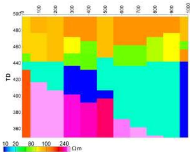
Figure 6. TD 1D inversion of data acquired from 4-layer model data.
