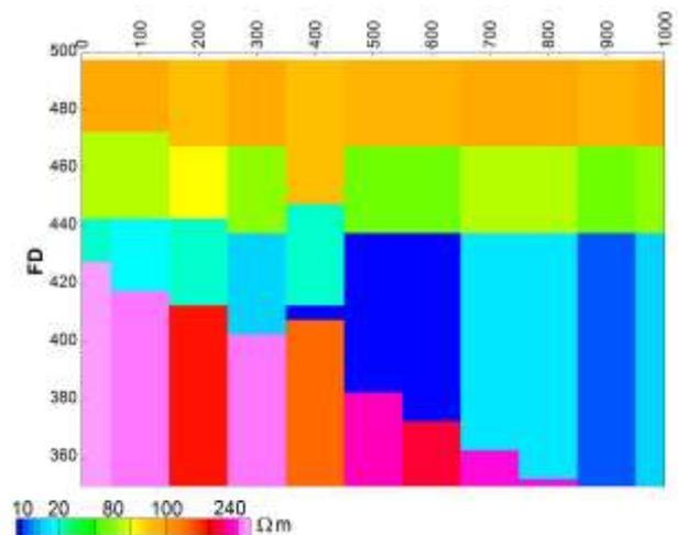
Figure 5. FD 1D inversion of data acquired from 4-layer model data.
