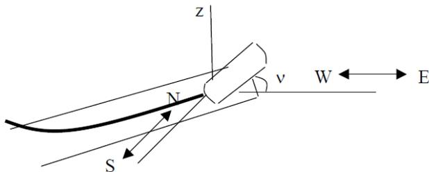
Figure 6. Inclined axis orientation in the W-E plane orthogonal to the horizontal projection of the magnetic field
