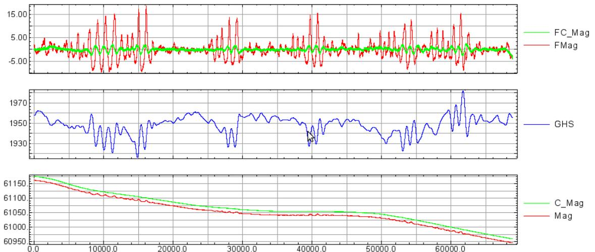
Figure 12. Compensation quality: F\_Mag — high-pass filtering results for non-compensated value, nT, FC\_Mag — high-pass filtering results for compensated value, nT, GHS — GPS altitude, meters, Mag — non compensated value, nT, C\_Mag — compensated value, nT, x axis shows fiducial for 100 samples per second
