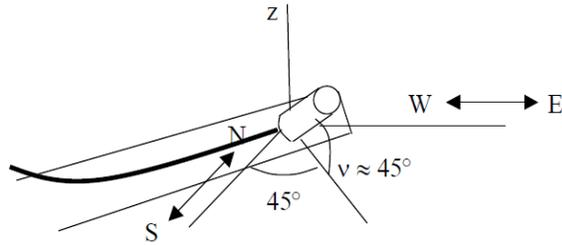
Figure 5. Inclined axis orientation
