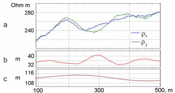
**Figure 1. Receiver positioning results: a) apparent resistivity calculated using actual bird position ( $\rho_1$ ) and using average offset ( $\rho_2$ ); b) vertical bird offset – affects  $\rho_2$  deviation about 10%; c) aircraft altitude – no influence on apparent resistivity**
