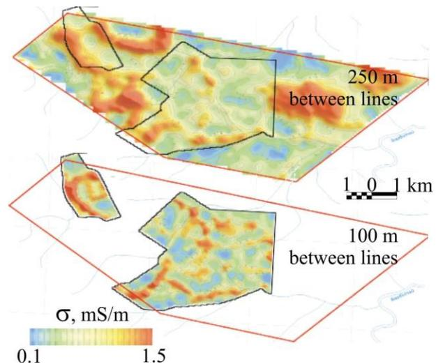
**Figure 4. Conductivity map after EQUATOR survey (upper image) and ground survey data (bottom image).**
