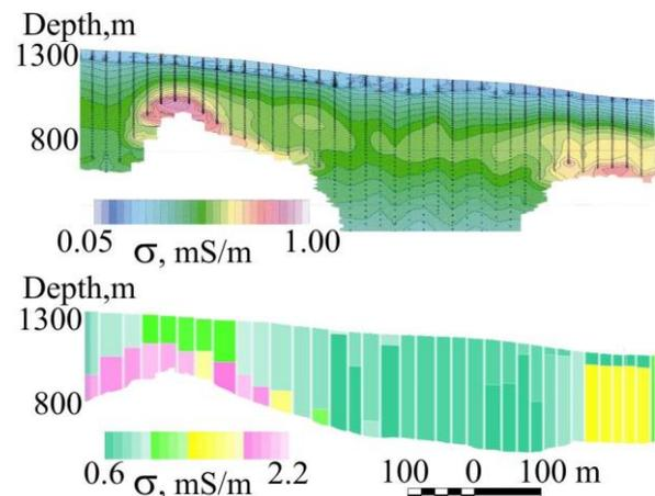
**Figure 5. Conductivity-depth image for ground survey data (upper image) and 2 layer inversion results (bottom image) for EQUATOR data over Ergoju deposits (deposits fit perfectly with conductive areas).**
